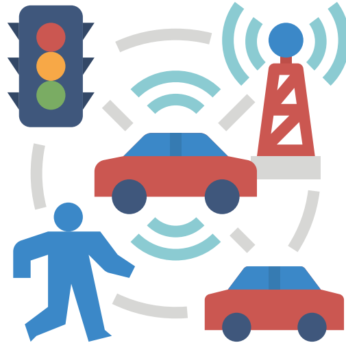
Figure 1: V2X (Vehicle-to-Everything) enables real-time communication between vehicles and their surroundings, including infrastructure, other vehicles, and pedestrians, to enhance safety and connectivity.
